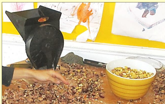
2. A DAVEBILT nut cracker is a hand-cranked device used for shelling thin-shelled nuts like pecans, hazels, and acorns. We have experimented with using it on dried chestnuts. Here we are shelling chestnuts after cracking them in the DAVEBILT.
